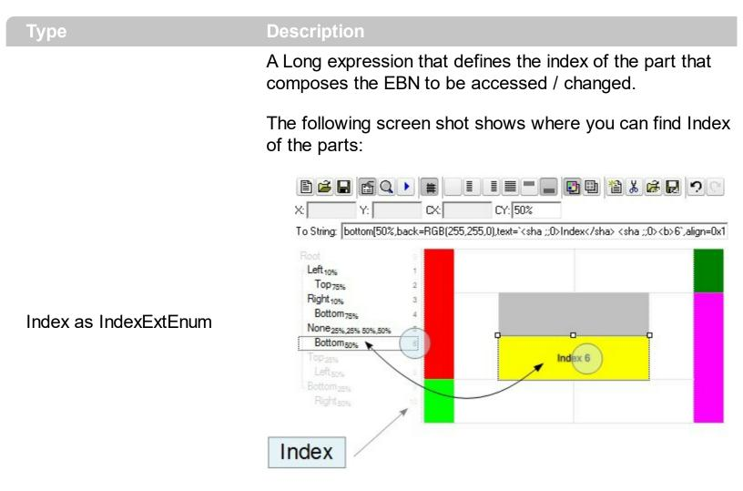
The screen shot shows that the EBN contains 11 elements, so in this case the Index starts at 0 (root element) and ends on 10.
